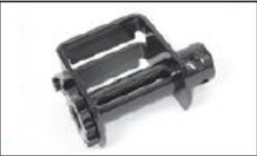
49207-187 Low Profile Double L Track Slider Lighter 7mm heat treated frame Weight: 6.2 lbs./2.8 kg. WLL: 5,500 lbs./2,500 kg.
