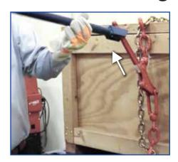
**Step 2:** Grip the Cobra Bar handle and pull up to release the tension of the load binder
