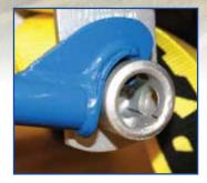
**Step 1:** Place the Cobra head securely into bar hole on winch cap
