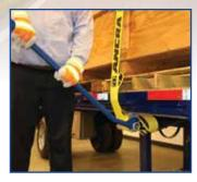
**Step 2:** Grip the knurled handle and pull down on the winch bar
