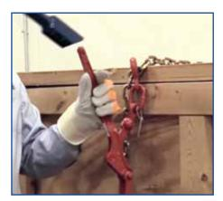
**Step 3:** Once the tension has been released, remove the box end from the load binder and continue removing the load binder as usual
