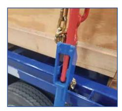
**Step 1:** Place load binder handle inside the combination box end of the Cobra Bar
