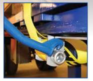
Step 3: Remove the Cobra Head from the current bar hole and resecure into the next bar hole available on the winch cap
